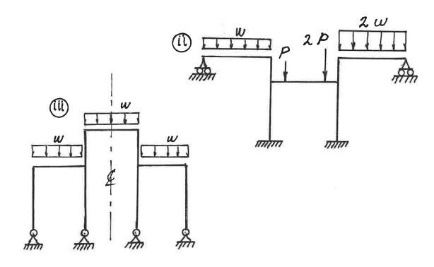
(12) Schematically show the shear force and bending moment diagrams for the following structures. All members have the same EI and are inextensible.
