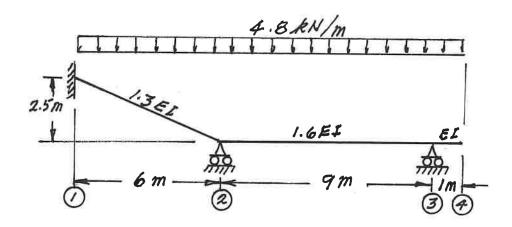
Using a **flexibility (force) method**, determine the moments at the ends of the fixed-ended, non-prismatic beam shown below. The relative EI values are shown.
