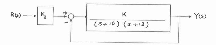
a) Determine the steady – state error for a unit step input in terms of K and  $K_1$ , where E(s) = R(s) - Y(s).
