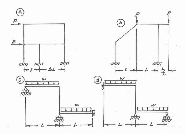
(12) 2. Schematically show the shear force and bending moment diagrams for the following structures. All members have the same EI and are inextensible.
