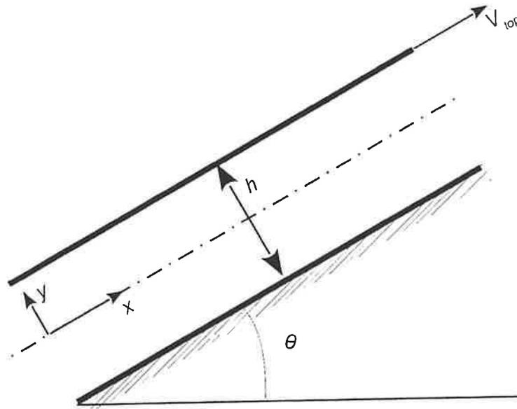
Figure 4: Inclined gravity and Couette driven flow.
