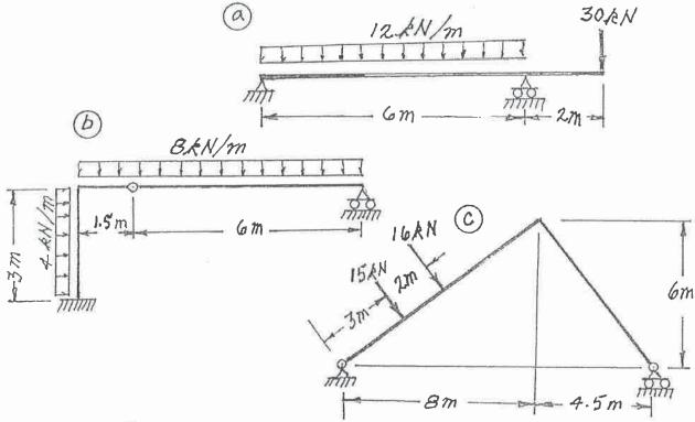
(16) 3. At point  $\bigcirc$  calculate the vertical deflection of the beam shown below. EI =  $2.7 \times 10^4 \text{ kN.m}^2$ .
