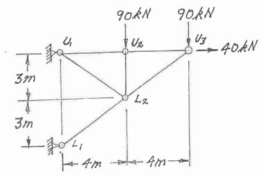
(9) 5. a) Loads move along beams at the top chord level of the truss shown below. Draw the influence lines for forces in members:
