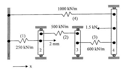
For the spring assemblage shown in the above figure,
