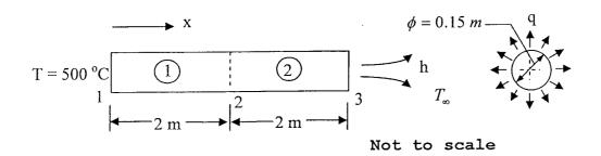
The thermal conductivity in the x-direction of the first and second element is  $K_{xx}^{(1)} = 300$  W/(m.°C) and  $K_{xx}^{(2)} = 600$  W/(m.°C), respectively. A uniform internal heat source  $Q^{(1)} = 400$  W/m³ is located in the first element and that in second element is  $Q^{(2)} = 500$  W/m³. Further, a uniform outgoing heat flux  $q_{out} = 10$  W/m² acts over the whole cylindrical surface of the rod.
