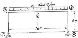
(22) 7. Using a flexibility (force) method, analyze the frame structure shown. All members have the same El value and are inextensible. Draw shear and bending moment diagrams. On both diagrams, for each member, indicate the magnitudes of the maximum and minimum ordinates (Minimum ordinates are frequently negative values.).
