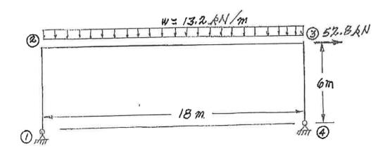
Using the slope-defection method or the moment-distribution method, analyze the frame structure shown below. Plot shear force and bending moment diagrams. For both diagrams, on each member label the magnitude of the maximum and minimum ordinates (Minimum ordinates are frequently negative values). All members are inextensible and have the relative EI values shown. Take advantage of symmetry.
