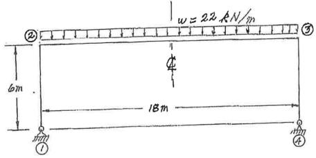
Use the moment-distribution method to analyze the structure shown. Draw shear and bending moment diagrams. On both diagrams, for each member, label the magnitudes of maximum and minimum ordinates (Minimum ordinates are frequently negative values). All members have the same EI value and are inextensible.
