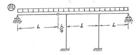
(11) 2. Schematically show the shear force and bending moment diagrams for the following structures. All members have the same EI and are inextensible.
