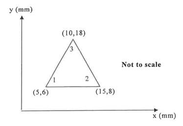
The nodal displacements for the plane strain element shown in the figure above are:  $u_1=0.003~\mathrm{mm}$  and  $v_1=0~\mathrm{mm}$ ;  $u_2=v_2=0~\mathrm{mm}$ ;  $u_3=0.005~\mathrm{mm}$  and  $v_3=0.003~\mathrm{mm}$ . The plate thickness  $t=0.6~\mathrm{mm}$ , and it is made from a material with Young's modulus of elasticity  $E=210~\mathrm{MPa}$  and Poisson's ratio v=0.3.
