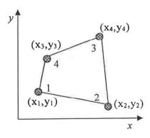
The shape functions of the element are given as
