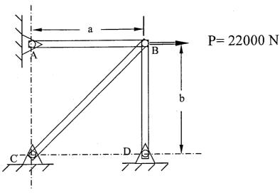
8- Determine the magnitude and direction (up or down) of the force P if the displacement at A is not to exceed 3 mm (down). Take E = 200 GPa and  $I = 805 \times 10^6$  mm<sup>4</sup>.
