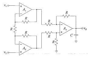
Given that all the op amps are ideal. The op amps' power supply is  $\pm 15$ V. Also, R = 10k $\Omega$  and C = 10µF.
