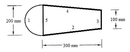
6- A stiffened thin walled wing box has a wall thickness t=2 mm and has been idealized into normal stress carrying booms 1 to 6 and shear only resisting thin wall panels. The box is subjected to a vertical force of 5,000 N acting upward as shown below. The boom areas are:  $B_1 = B_6 = 500 \text{ mm}^2$ ,  $B_2 = B_5 = 300 \text{ mm}^2$  and  $B_3 = B_4 = 800 \text{ mm}^2$ .
