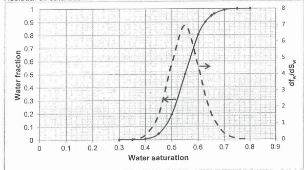
a) Estimate cumulative oil production when water saturation at the production wells is 66%
