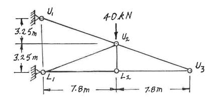
(18) 4. For the trusses shown below, calculate the forces in the members that are listed. For each force, indicate whether it is tension or compression.
