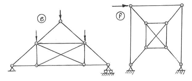
(22) 2. For each structure shown, compute the reactions and draw shear and bending moment diagrams. Indicate which are positive and which are negative segments of each bending moment diagram. For each shear and bending moment diagram, calculate and indicate the magnitudes of the maximum positive and negative ordinates.
