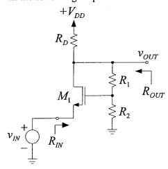
a) Determine the input and output resistance ( $R_{IN}$  and  $R_{OUT}$ ) if there is no feedback network (i.e.  $R_1 = \infty$ , and  $R_2 = 0$   $\Omega$ ).
