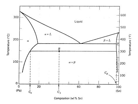
Figure 1 – Pb-Sn phase diagram.
