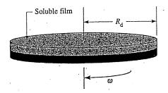
A solid disk rotates about an axis normal to its circular face and is immersed in a large volume of fluid. Except for the motion induced by the rotation of the disk, there is no imposed convective flow in the system. The surface of the disk is coated with a solid film of a material that is soluble in the surrounding fluid. A significant motion is induced by the rotation of the disk, and this motion gives rise to significant convective mass transfer from the disk surface.
