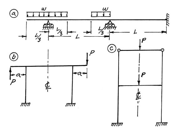
(8) 2. For the beam structures shown below, schematically show the influence lines for shear forces immediately left of support  $\bigcirc$ . Note that structure a) is determinate and b) is indeterminate. Show the value of the ordinate with the maximum absolute value on each influence line.
