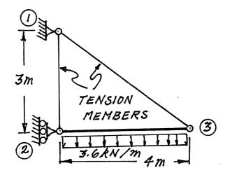
(18) 4. Use Castigliano's first theorem (the least work theorem) to analyse the structure shown. Calculate the maximum bending moment in the horizontal beam. All three beams are inextensible and have the relative EI values shown; for beam 2-3 the value of EI = 9280 kN.m<sup>2</sup>. The tension member has EA= 1900 kN. To minimize calculations, take advantage of the symmetry.
