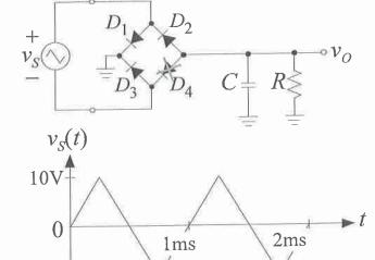
Due to an abnormal operating condition, Diode  $D_4$  in this full-wave rectifier circuit was suddenly destroyed, and stopped conducting in both forward and reverse directions (i.e. open circuit).
