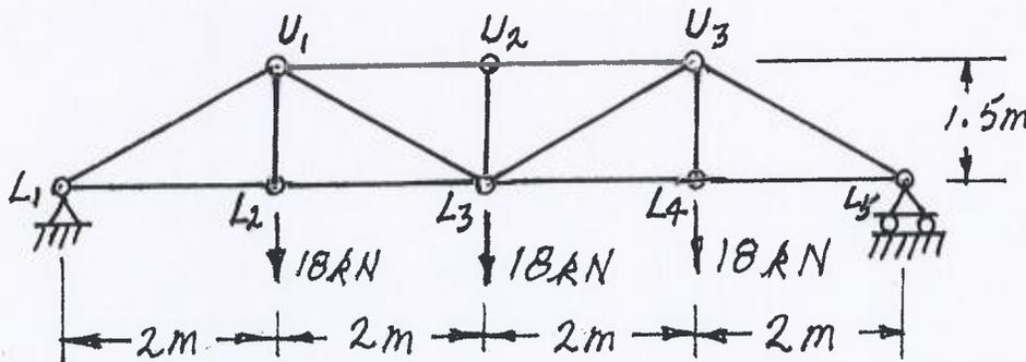
(18) 4. For the trusses shown below, calculate the forces in the members that are listed. For each force, indicate whether it is tension or compression.
