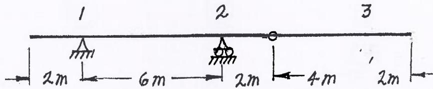
b) A vehicle, which is idealized as the three point loads spaced as shown below, moves on beams at the bottom chord level of the truss shown. The shape of the influence line for force in member  $U_1 - L_3$  is shown below the truss. Calculate and show the ordinates of the influence line and calculate the maximum force caused by the vehicle as it crosses the structure.
