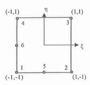
(a) [14 marks] Determine the shape functions ( $N_i$ , i = 1 to 6) of the six-node transition element in natural/local coordinates ( $\xi, \eta$ ) such that  $-1 \le \xi, \eta \le 1$ .
