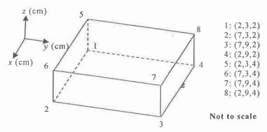
(a) [4 marks] Determine the shape functions ( $N_i$ , i = 1 to 8) of an eight-node hexahedron element in natural/local coordinates ( $\xi, \eta, \zeta$ ) such that  $-1 \le \xi, \eta, \zeta \le 1$ . The node numbering is identical to that shown in the above representative global element.
