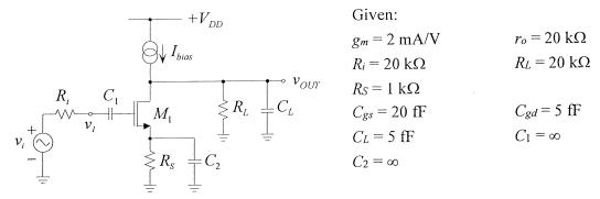
d) Find the mid-band voltage gain  $v_{OUT}/v_i$ .
