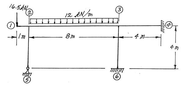
(22) 7. Use the **principle of virtual work** to calculate the vertical deflection at point 4 on the frame structure shown below. All members are inextensible and have the same EI value which is 2,000 kN.m<sup>2</sup>.
