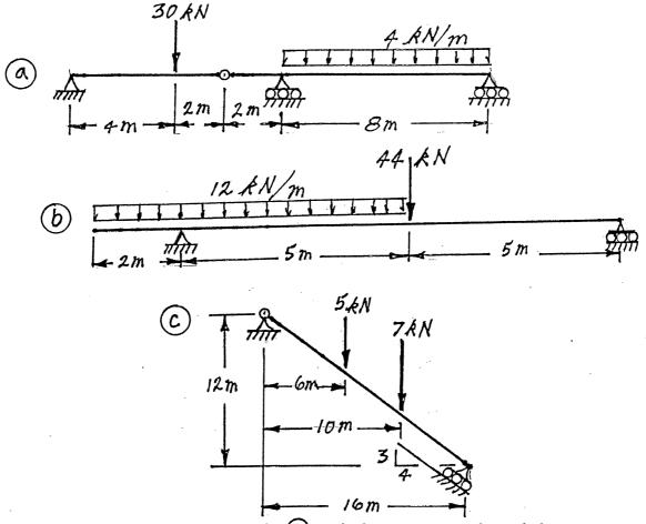
(15) 3. Calculate the vertical deflection at point B on the beam structure shown below. EI = 15,000 kN.m<sup>2</sup> for all spans.
