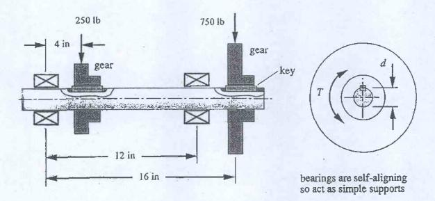
**Problem 4.** A journal and bearing are to be designed for a shaft that turns at 250 rpm. Suppose ISO VG100 (SAE Engine 30) is to be used as lubricant and the bearing length is to be equal to 1.2 times the diameter. If the no-load power loss is not to exceed  $2.5 \times 10^{-4}$  horsepower and the diametral clearance is 0.0045 times the diameter, estimate the maximum diameter that can be used for the journal, and the allowable temperature limit. (20 marks)
