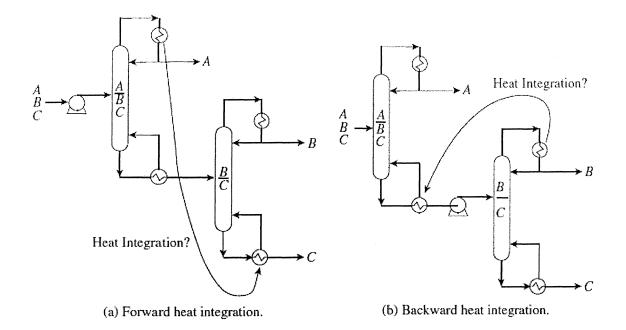
The operating pressures of the two columns need to be chosen to allow heat recovery. Data for Column #1 and Column #2 at various pressures are given below:
