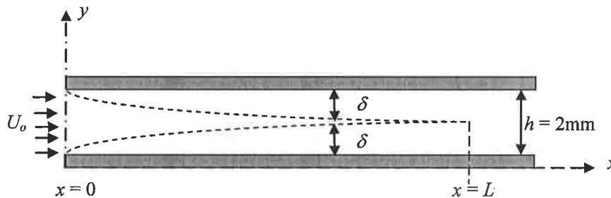
**Figure Q4:** Schematic of two-dimensional inlet region.
