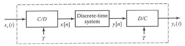
The input signal  $x_c(t)$  has the Fourier transform shown in the figure below with  $\Omega_0 = 2\pi(1000)$  rad/s. The discrete-time system is an ideal lowpass filter with frequency response
