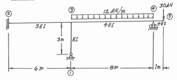
Use the principle of virtual work to calculate the horizontal deflection at point  $\Im$  on the structure shown below. Consider only flexural strain. All members are prismatic and have the same EI value; EI =  $2.0 \times 10^5 \text{ kN.m}^2$ .
