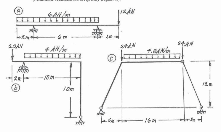
(18) 3. Calculate the vertical deflection at point ② on the continuous beam shown below.  $EI_0 = 9000 \text{ kN.mm}^2$ .
