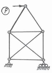
(18) 2. For each structure shown, compute the reactions and draw shear and bending moment diagrams. Indicate which are positive and which are negative segments of each bending moment diagram. For each member on the shear and bending moment diagrams, calculate and indicate the magnitudes of the maximum and minimum ordinates (Minimum ordinates are frequently negative.).
