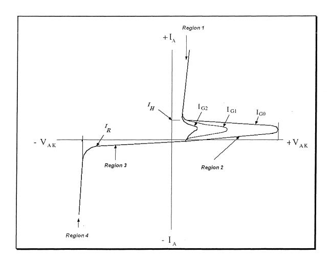
Figure (1) SCR Characteristics
