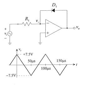
The op amp in this circuit is ideal except for a slew rate limit of  $0.5V/\mu s$ . It is powered by  $\pm 15V$  supplies. Given that
