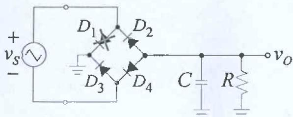
Due to an abnormal operating condition, Diode  $D_1$  in this full-wave rectifier circuit was suddenly destroyed, and stopped conducting in both forward and reverse directions (i.e. open circuit).
