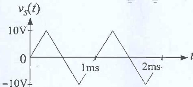
Assume that all other diodes are ideal with zero forward voltage drop and that the time constant  $RC = 5\text{ ms}$ . For a  $1\text{ kHz}$  triangular input waveform with a peak amplitude of  $10V$ ,
