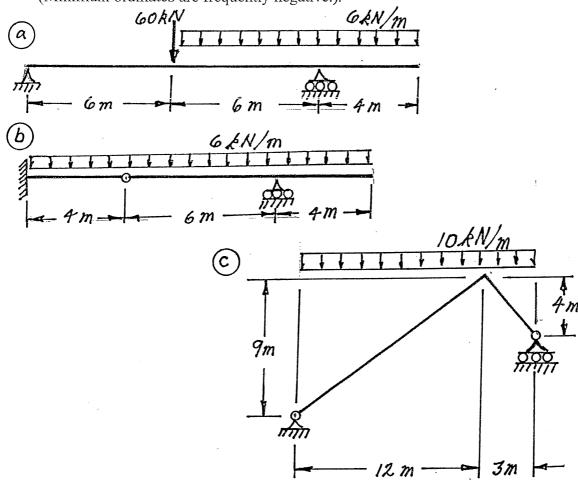
(18) 3. Calculate the vertical deflection at point  $\triangle$  on the continuous beam shown below. EI = 2000 kN.m<sup>2</sup> for all beam segments. Take advantage of symmetry.
