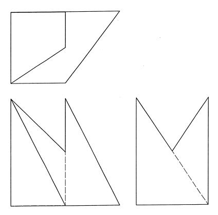
3. Draw the oblique face(s) of the below component in true shape. Show all work. Clearly label the auxiliary view. Complete the answer in the space provided below.
