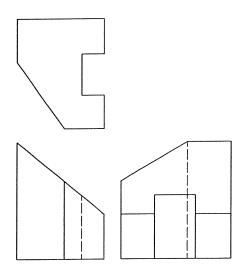
4. Fully dimension the follow orthographic projection using Canadian conventions (CSA/ANSI) in inches. The component is drawn in half scale. Complete the answer on the drawing provided.
