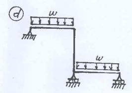
(12) 2. Schematically show the shear force and bending moment diagrams for the following structures. All members have the same EI and are inextensible.
