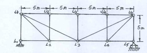
Use the slope-defection method to analyze the frame structure shown. Draw shear and bending moment diagrams. Indicate on both diagrams the magnitude of maximum and minimum ordinates. There are no loads on the structure, but pin-ended columns 1-5 and 4-8 were both fabricated 0.048 m too long; the columns were forced into place. All members of the structure have the same EI value that is 5.0 x 10<sup>4</sup> kN.m<sup>2</sup> and all members are inextensible.
