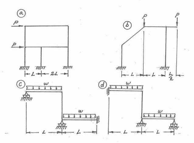
Schematically show the shear force and bending moment diagrams for the following (12)2. structures. All members have the same EI and are inextensible.
