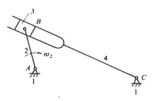
(iv) The input link moves at a constant linear velocity of 10 m/s in the direction shown in the below figure. When the follower is pushed to rotate 30 degrees clockwise (CW) from its initial vertical position, determine (the angular velocity and angular accelerations of the follower.
