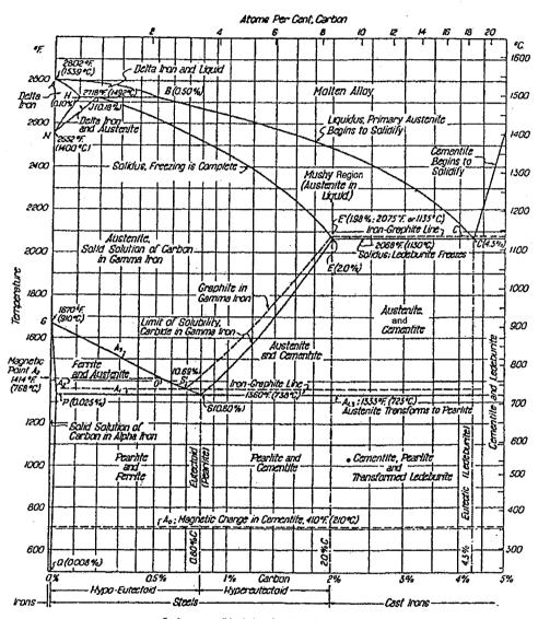
Ferrite = solid solution of carbon in lower temperature, body
