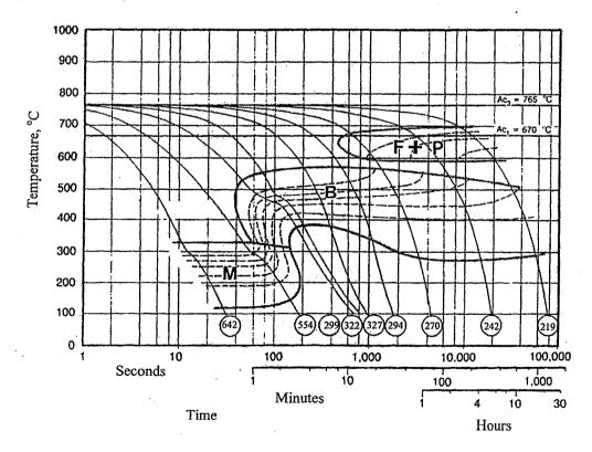
Considering the TTT diagram for a hypo-eutectoid steel, presented in the Figure above, calculate the cooling rates needed, in order to obtain 1) a F+P (ferrite and
