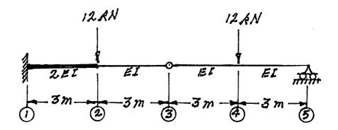
(16) 5. Analyze the structure shown below using the slope-deflection or moment-distribution method; calculate and plot the shear force and moment diagrams. On each diagram for each member, label the maximum and minimum ordinates (Minimum ordinates are frequently negative values). All members have the same EI and are inextensible.
