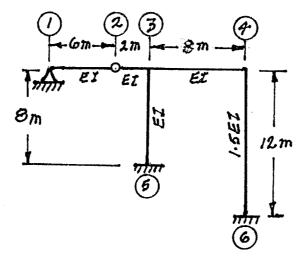
Using a **flexibility (force) method**, analyze the frame structure shown. Both members have the same EI value and are inextensible. Draw shear force and bending moment diagrams. For each member, on each diagram indicate the magnitudes of the maximum and minimum ordinates (Minimum ordinates are frequently negative values).
