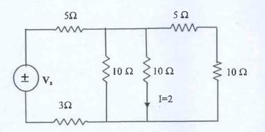
**Q1(B):** Find Thevenin equivalent circuit at terminals a-b of the circuit shown below . [6]What load  $R_L$  should be connected to a-b in order to get maximum  $P_L$ ?[2]Calculate the maximum power which can be transferred to  $R_L$ .[4]
