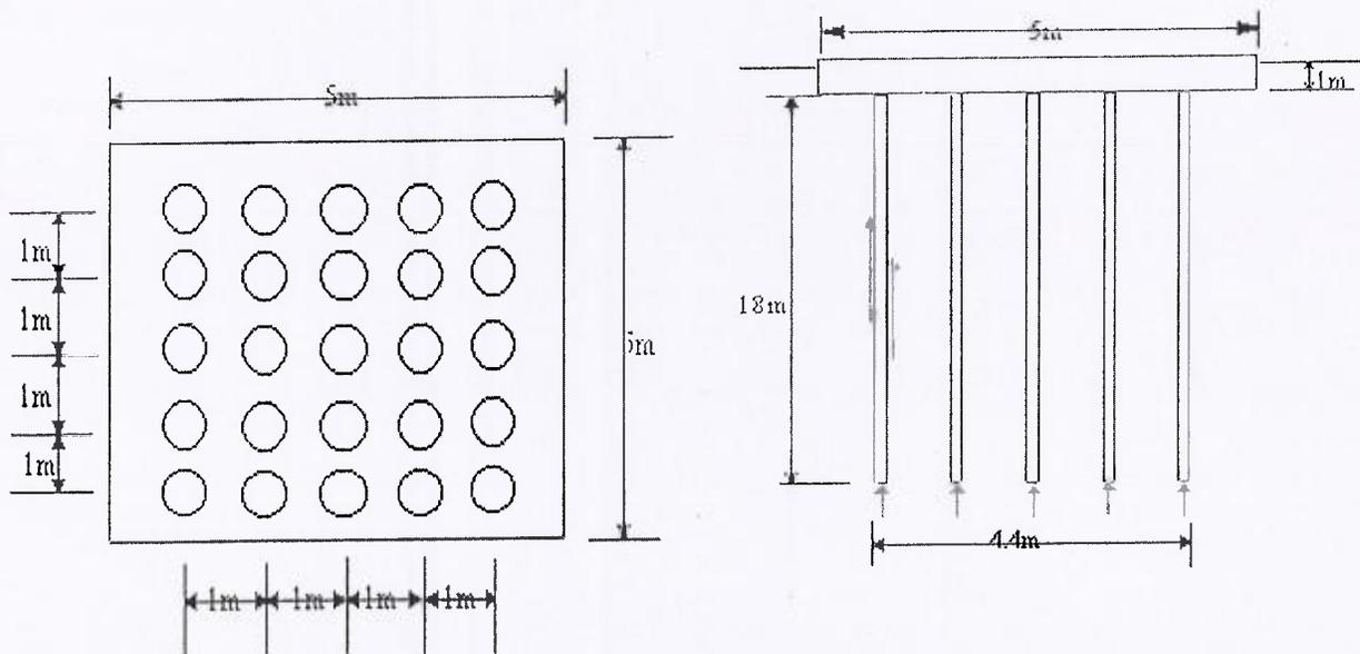
Figure for Question 5: a) Plan view; b) elevation view
