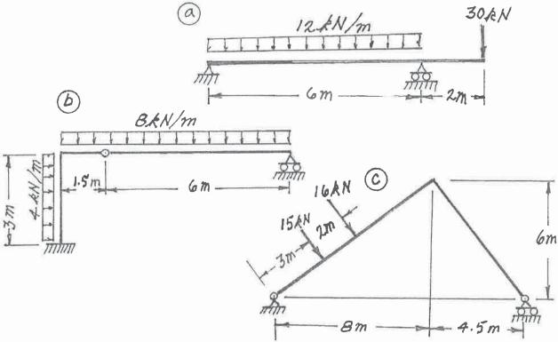
(16) 3. At point  $\bigcirc$  calculate the vertical deflection of the beam shown below. EI =  $2.7 \times 10^4 \text{ kN} \cdot \text{m}^2$ .
