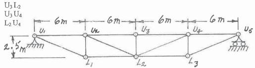
For each influence line, calculate and indicate the value of the influence ordinate at the  $\frac{1}{4}$ ,  $\frac{1}{2}$  and  $\frac{3}{4}$  points along the truss span.
