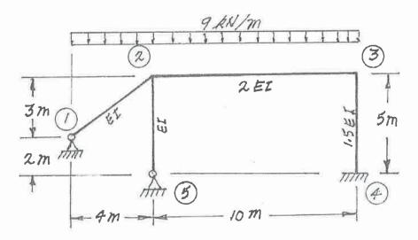
Use the principle of virtual work to calculate the vertical deflection at point © on the structure shown below. Both beam members are inextensible and their relative EI values are shown on the diagram; EI = 3500 kN.m<sup>2</sup>. For the strut, AE = 25000 kN.
