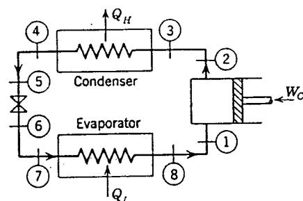
The heat transfer from the Freon-12 during the compression process is 4 kJ/kg. Sketch the various processes on a temperature-entropy diagram and determine the coefficient of performance of the cycle.
