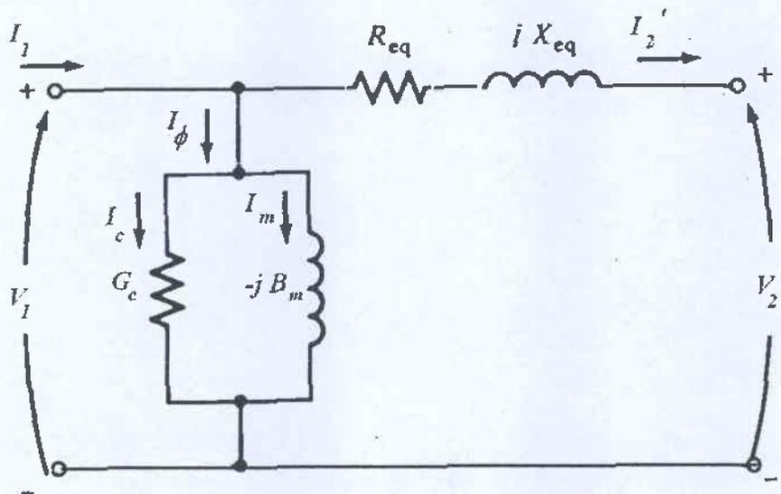
Figure (1) Equivalent Circuit of Transformer for Problem 3
