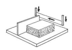
smooth finish to that side. After each cut the operator manually turns and re-aligns the stack against the stop for the next cut on another side.
