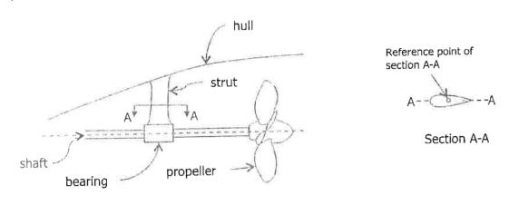
(a) Shaft, bearing, strut and propeller in profile. (Strut cross-section shown on the right hand side)
