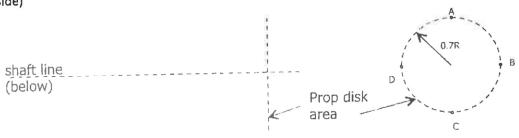
(b) 4 points in the propeller disk area at the 0.7R radius fraction shown at right.
