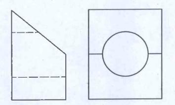
4. Dimension the following orthogonal projection using Canadian conventions (CSA/ANSI) in millimetres. Add centre lines and centre marks as needed. The component is drawn in full scale. Complete the answer on the drawing provided.
