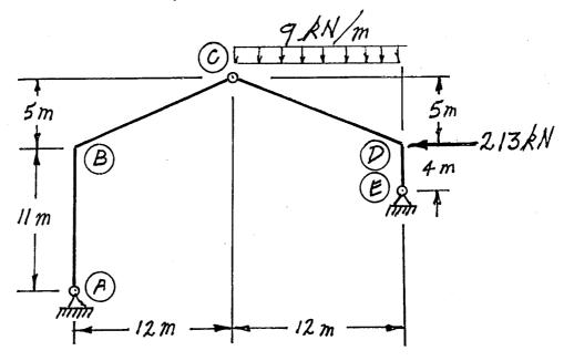
Using the principle of virtual work, calculate the horizontal deflection at point  $\bigcirc$  of the structure shown below. The tie rod has an AE =  $4.5 \times 10^4$  kN. Both beams are inextensible and have EI =  $2.4 \times 10^5$  kN.m<sup>2</sup>.
