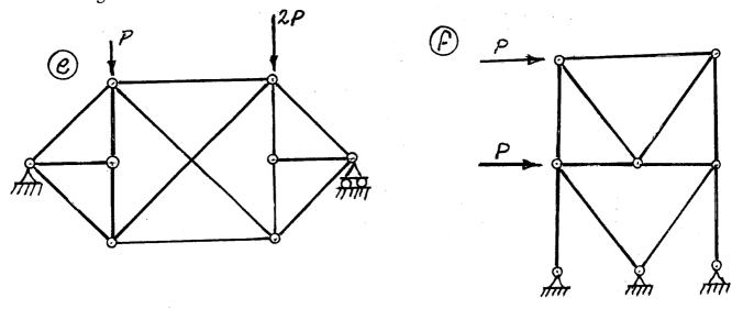
For each structure shown, compute the reactions and draw shear and bending moment diagrams. Indicate which are positive and which are negative segments of each bending moment diagram. For each shear and bending moment diagram, calculate and indicate the magnitudes of the maximum positive and negative ordinates.
